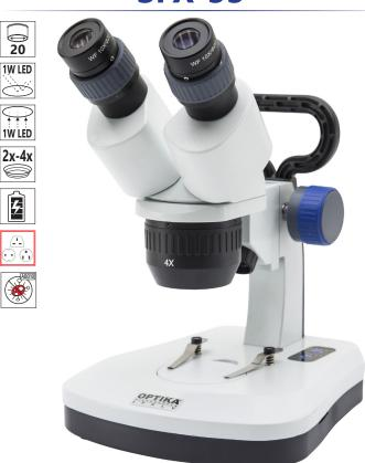
Cordless binocular stereomicroscope ideal for students, schools and amateurs to dissect and discover mainly biology and materials science in 3D, with turnable objective (2x-4x), FN 20 eyepieces, fixed arm with handle and 1 W LED transmitted / incident illumination with comfortable touch control and rechargeable batteries. Slim and easy to carry, it is equipped with long lasting LED illumination to provide over 20 years of
